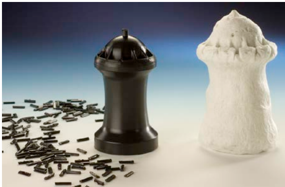
Fig. 4: Pictured left, the ten millimetres long glass fibre granules and the black test part reinforced with long glass fibres. To the right, the fibre felt structure remaining after ashing of the test part at high temperatures.
